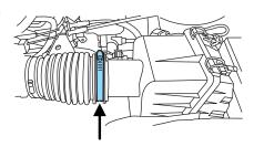
12. Reconnect the Mass Air Flow Sensor electrical connector to the outlet tube. Make sure the locking tab on the connector is in "locked" position.
